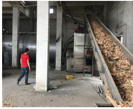
5) 3.0million kcal biomass gasifier connect to 5-ton vertical boiler in Thailand (replace firewood)
