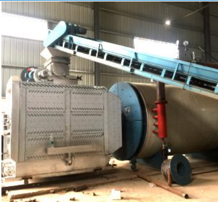
4) 3.6 million kcal biomass gasifier connect to Hengyang glycerin production plant 3500kw thermal oil boiler
