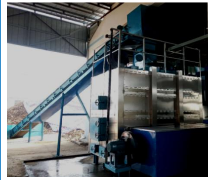
6) 3.6 million kcal biomass gasifier connect to Zhaoqing Xinqiao Food & Beverage Factory's 6-ton hand-fired boiler(replace coal)
